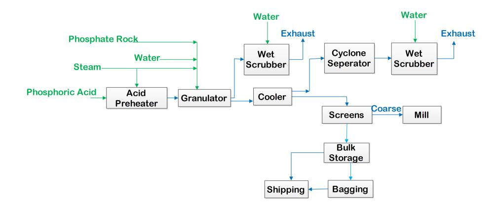
Figure: Manufacturing of Triple Superphosphate
